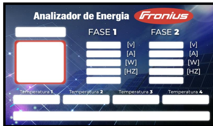
Figura 3.12: Pantalla principal HMI
